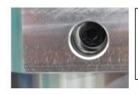
Tighten the clamping screw in the clamping hub with suitable MA,
