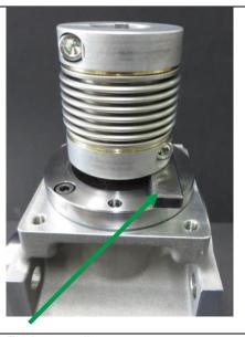
Fit the coupling, prepare as described above. If prescribed, adjust the assembly dimension of the coupling according to the dimension sheet.
