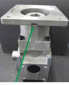
Install the lantern and tighten the screw(s). The coupling can be tightened on the motor side through the hole at the top. It is recommended to turn the lantern so that this hole is on the side of the terminal box of the motor.
