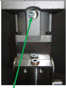
Install the lantern and tighten the screw(s). The coupling can be tightened on the motor side through the hole at the top.
