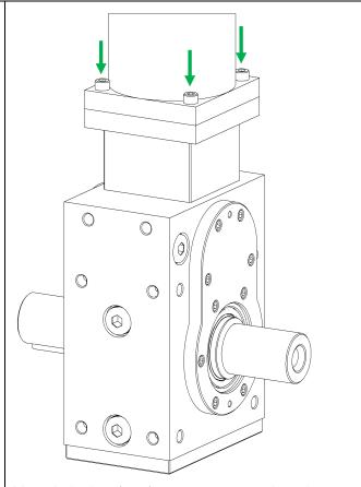
Motor bolted on free from any stress and tension (pictured: KS FL)
