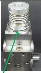
Fit the coupling, prepare as described above. If prescribed, adjust the assembly dimension of the coupling according to the dimension sheet.
