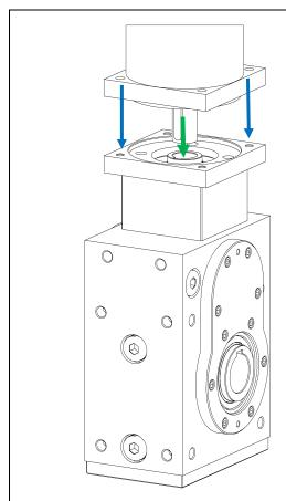
Motor mounting vertically from the top (pictured: KS FH), define position of the terminal box, then join up motor, with the key on the motor in alignment with the key groove in the shaft, then continue as described above.
