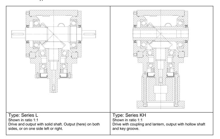
Shaft bearings with angular contact ball bearings, lubrication with synthetic gear oil ISO VG 150
