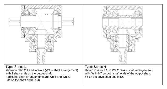
The bearings are designed with tapered roller bearings. The drive pinions are shrunk into the driven pinion gears on the shaft. In case of the **reinforced X version**, the drive shafts are designed as pinion shafts.
