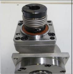
Fit the coupling and prepare as described above. If specified, set the mounting dimension of the coupling in accordance with the dimension sheet. Tighten clamp screw.
