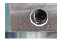
Tighten the tensioning screw in the clamping hub with a suitable M<sub>A</sub>,
