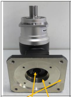
Clean the clamping hub, bore and flange surface of the planetary gear stage so that it is free of dirt and grease and then do the same on the motor shaft and motor flange.
