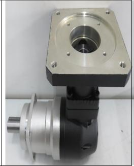
The motor must be in tension-free contact with the gearbox flange, then screw in screws using screw locking paste and tighten crosswise to the prescribed tightening torque.
